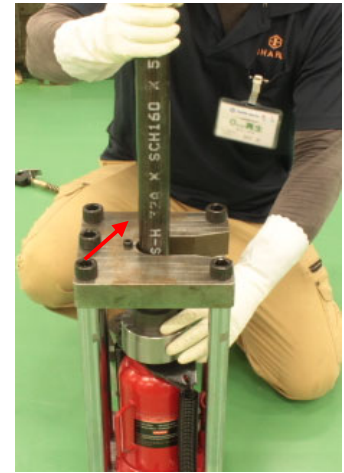
④ While supporting the components and preventing them from falling, insert the tube into the U-shaped flange, reaching the back. Place it on top of the hydraulic jack. In this position, the core of the jack and the components align.
