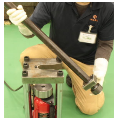
⑥ Gently open the relief valve of the hydraulic jack, return the cylinder to its original position, and remove the tube assembly.
