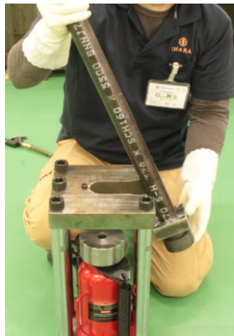
④ While supporting the components and preventing them from falling, insert the tube into the U-shaped flange, reaching the back. Place it on top of the hydraulic jack. In this position, the core of the jack and the components align.
