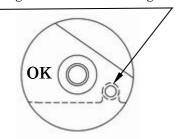
There is a gap between the locating pins and the grooves in two places.
