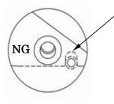
When there is a gap between the hole and the tap, the cutter blade holder cannot be set to the proper position. In such case check for foreign matter such as chips being caught.
