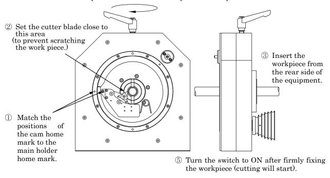
Precaution: When a long tube is to be cut, provide supports before and after the collet to hold the tube approximately horizontally.
