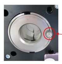
Match the position of the collet notch to the tap hole position, and then insert the collet.
