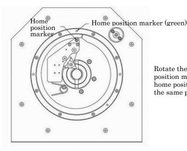
Rotate the cam until the cam home position marker and the main holder home position marker match and are at the same position.
